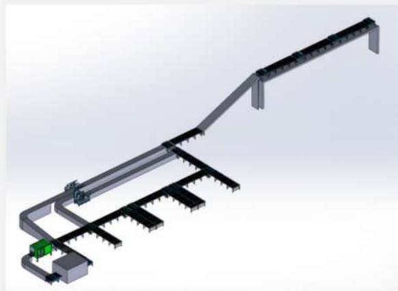
Sorting line of light vehicle and truck tyres granulator. Application : material recovery.
